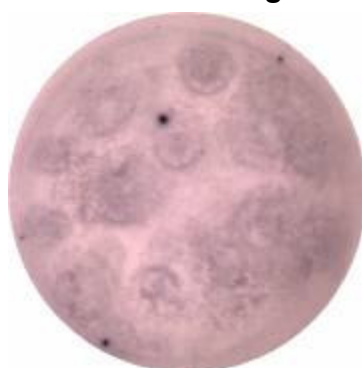
Plate was not thoroughly rinsed after developing and then dried flat: Residual color forms structures
