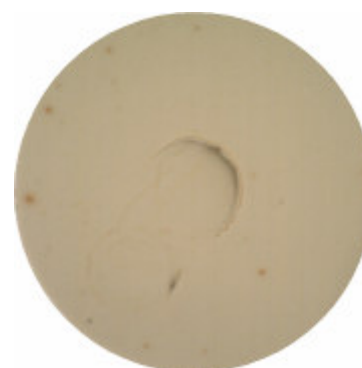
Pipet tip has pierced the membrane
